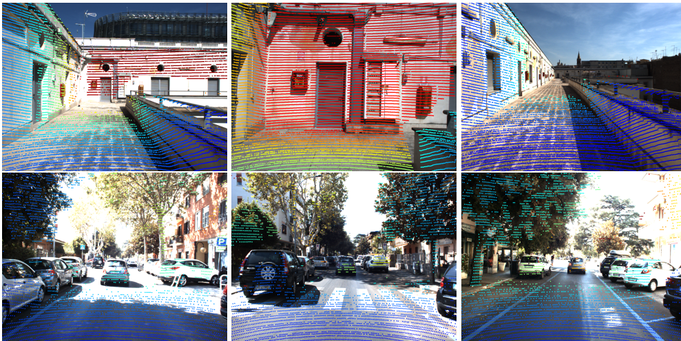
Figure 5.3. Qualitative samples showing LiDAR cloud projection on RGB image.
