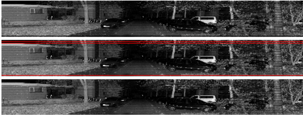
Figure 3.2. Empty lines removal. From top to bottom, original image after projection from 3D point cloud as explained in Sec. 3.2.1, detection of empty rows highlighted in red, result after image manipulation. Each image shown has been cropped to half of their horizontal size for better viewing.
