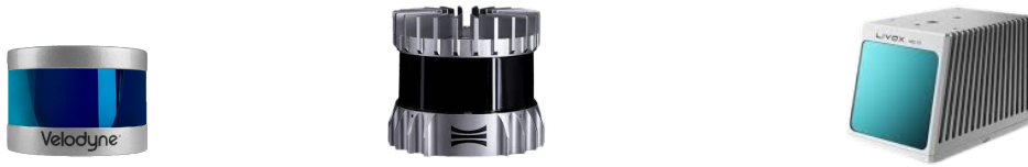
Figure 2.5. Different LiDARs available in the market. From left to right respectively Velodyne Puck [7], Ouster OS-128 [6] and Livox MID-70 [4]. Velodyne Puck, often referred to as the VLP-16, is a mechanical LiDAR equipped with 16 laser channels and is commonly used in various applications from drones to robotics due to its balance of performance, size, and price. It provides a 360 deg horizontal FoV and a vertical one of roughly 30 deg. Ouster OS-128 is always a mechanical LiDAR but with higher vertical resolution, as its name implies, it has 128 laser channels, offering a denser point cloud which is crucial for applications that require intricate detail. While the horizontal FoV is always 360 deg due to encoder rotation, its vertical FoV can reach up to 90 deg. It is the one we have used more in our work, due to its higher vertical capabilities. Livox MID-70, on the other hand, is a solid-state LiDAR and differentiates itself with its non-repetitive scanning pattern. Unlike traditional mechanical LiDARs that scan in a set, predictable pattern, Livox employs a unique approach where the scanning pattern is more random, aiming to achieve more uniform point cloud distribution.
