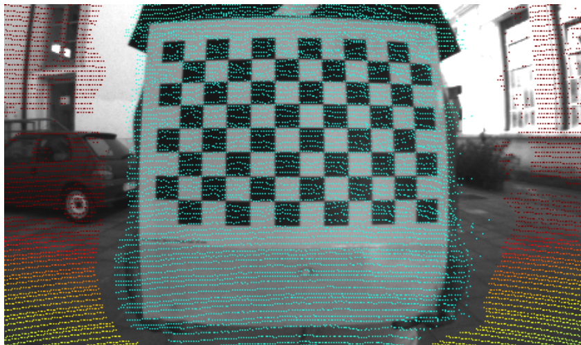
Figure 5.1. Camera/LiDAR qualitative calibration results. The image shows the reprojection of a LiDAR point cloud on a image captured by a fisheye RGB camera rigidly attached to the former. The offset between the sensors leads to shadows on parts of the image.
