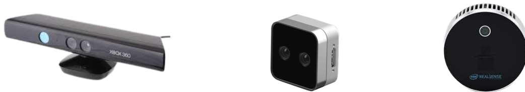
Figure 2.2. Different depth cameras. From left to right respectively Microsoft Kinect [5], Intel D405 [3] and Intel L515 [2]. Kinect, initially designed for gaming, utilizes both infrared and RGB cameras. It primarily leverages structured light technology, projecting a specific pattern onto a scene measuring the difference of the calibrated pattern to estimate depth. With its baseline of around 7 cm can reconstruct depth til 6/7 meters. Differently D405, does not rely on IR emitters, it is just equipped with two global shutter cameras and with its really small baseline is capable to reconstruct depth at sub-millimeters accuracy at an ideal range of 7 cm (till a maximum one of 50 cm). The one on the right, L515, is a depth camera that relies on ToF technology. As for LiDAR the good thing about active depth sensing is its capability to work in various lighting conditions, including total darkness. Its maximum depth is of 7 meters.
