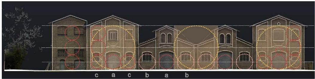
drawings with the current survey of the building there is a remarkable correspondence (fig. 8), thus providing a tangible demonstration of the accuracy and reliability of the metric data contained in the historical drawings.
