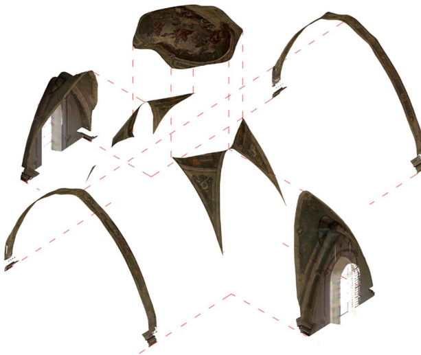
Fig. 3 Exploded axonometry of the architectural elements that make up the vault covering each bay
