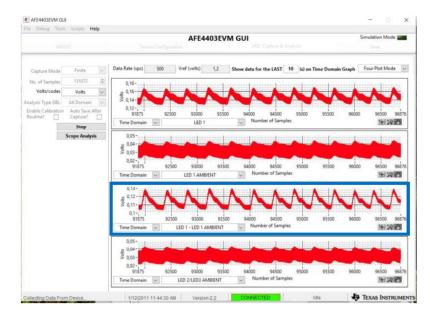
**Figure 9.** ADC Capture & Analysis section of the AFE4403EVM sensor GUI. The blue box indicates the channel in which the ambient light is subtracted from the signal (LED1-LED1 AMBIENT).
