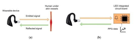
Figure 3. Scheme of the conventional use of a PPG device (a) and the one proposed in this paper (b).
