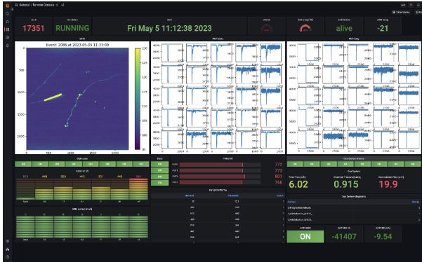
Figure 3. The CYGNO remote console available for user following the run from remote - without the need to access the DAQ, restricted to experts - where the following are available: device setting and readout, sample of raw images collected and PMT waveforms, typically updated every 5 seconds.
