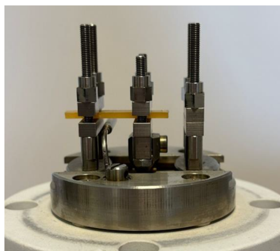
Figure 3. DMA-1 in single cantilever configuration: front view.
