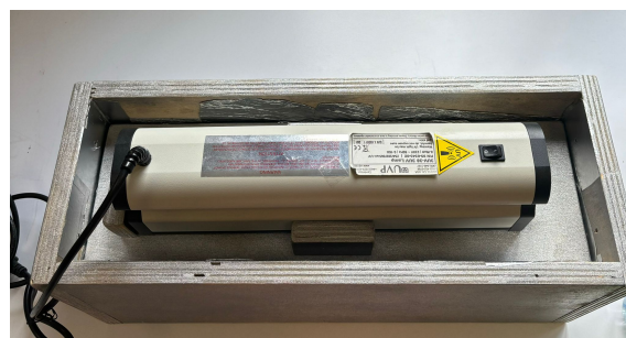
Figure 1. Low-pressure UV lamp used for the UV-C irradiation process in laboratory.
