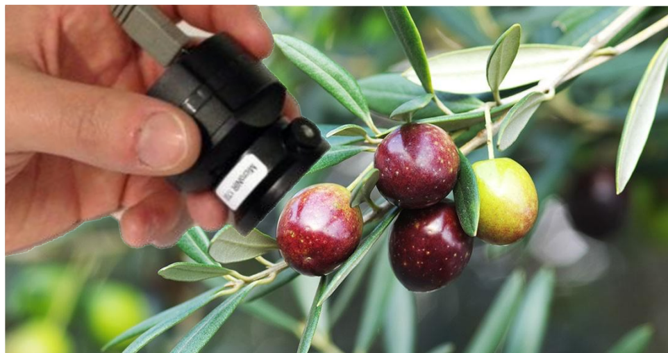
Figure 1. Acquisition of spectra of olives by the MicroNIR.
