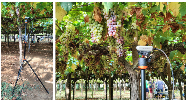
Fig. 3: Experimental setup for data acquisition, a Intel RealSense d435i camera mounted on a tripod for stabilization during movements.
