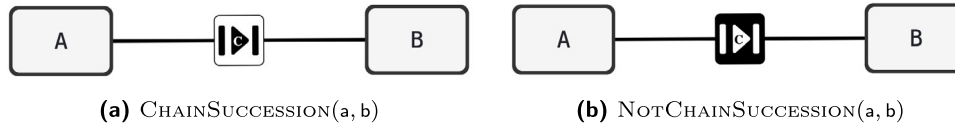
Fig. 5. An example of a \text{CHAINSUCCESION}(a, b) and a \text{NOTCHAINSUCCESION}(a, b) . The white background (a) and black background (b) on the constraint symbol discriminate between a positive and a negative relation.
