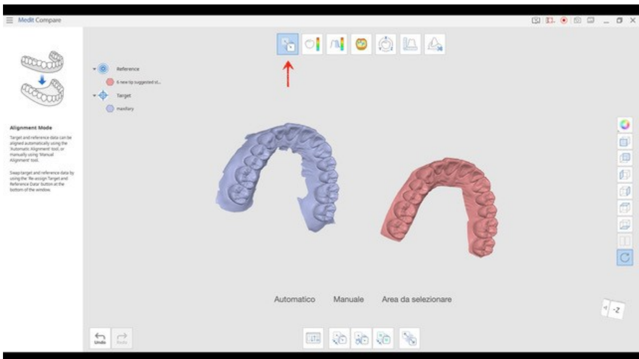
Figure 4. The STL file of the RG and that of the TG were uploaded into the software. The arrow indicates the tool to be used for the alignment of the two STL files.
