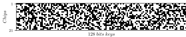
Fig. 9. Graphical representation of the 128-bits PUF keys on all the 20 chip samples.
