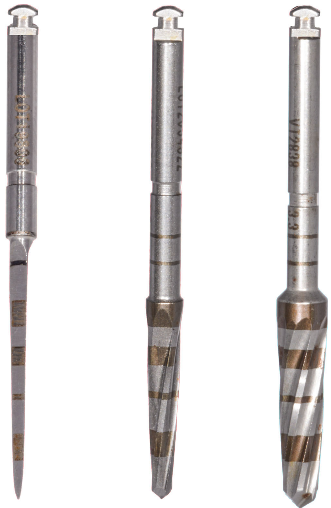
FIGURE 1 Osseodensification drills (Densah, Versah) were used at 1200 rpm in the following sequence: from left to right (I) pilot (clockwise); (II) WT1828 (counterclockwise), and (III) WT2838 (counterclockwise).
