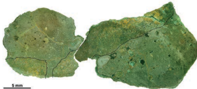
Figure 6.14: Polished sections of the two fragments comprising 220-2242. The borders between areas with different microstructures are indicated by dotted lines.
