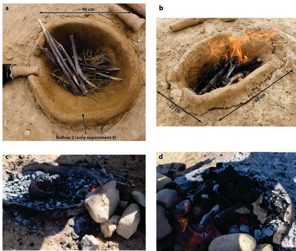
Figure 5.3: The furnaces used in the experiment to fire the moulds: (a) The furnace to melt the metal in a crucible before kindling the fire; the later position of bellow 2 is indicated. (b) The furnace for de-waxing; (c) The location of the moulds from experiment 1 to 3 in the furnace for wax removal; (d) The crucible furnace with the mould from experiment 4 placed between the tuyères. The tuyères are located under the cobble stones.
