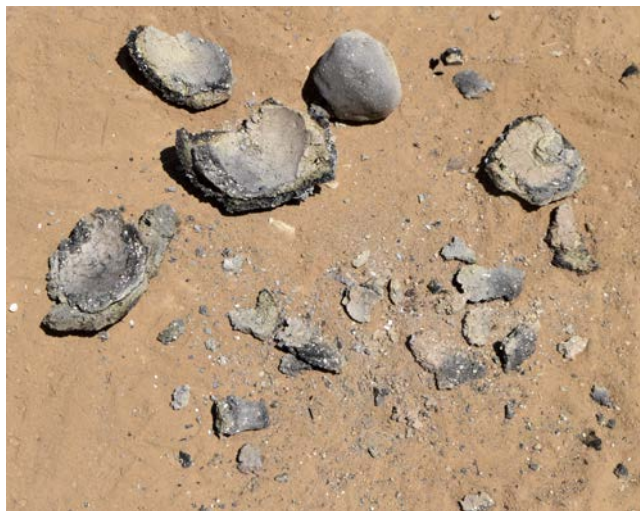
Figure 5.5: The mould of experiment 1 after it was accidentally broken in the field. The separation of layers 2 and 3 is especially clear at the larger fragments.
