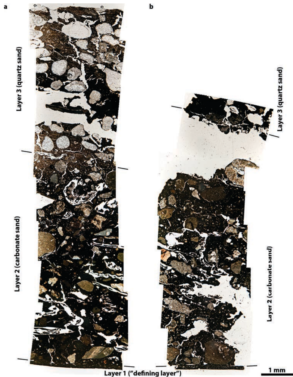
Figure 5.9: Cross sections through (a) the complete mould of experiment 3 (Exp3-M3); (b) the mould of experiment 4 with layer 3 detached during sampling and the outer part of layer 3 missing (Exp4-M3). The approximate locations of the interfaces between the layers are indicated. Composite images.
