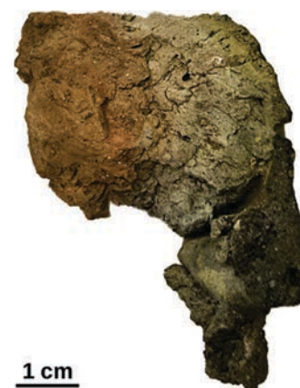
Figure 6.15: Furnace wall fragment A-F-10 with ceramic melt solidified in a flow texture with bulges.
