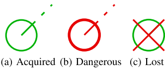
Fig. 1. ARPA target symbols on the PPI.
