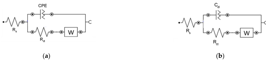
Figure 6. Equivalent circuits used for fitting the experimental data: circuit (a) for h-nPG modified electrode and Au/SWCNTs modified electrode (Randles circuit), and circuit (b) for Au bare electrode.
