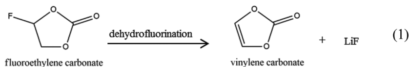
Scheme 1. Dehydrofluorination reaction of FEC generating VC and HF, which further reacts with Li ions leading to LiF formation.
