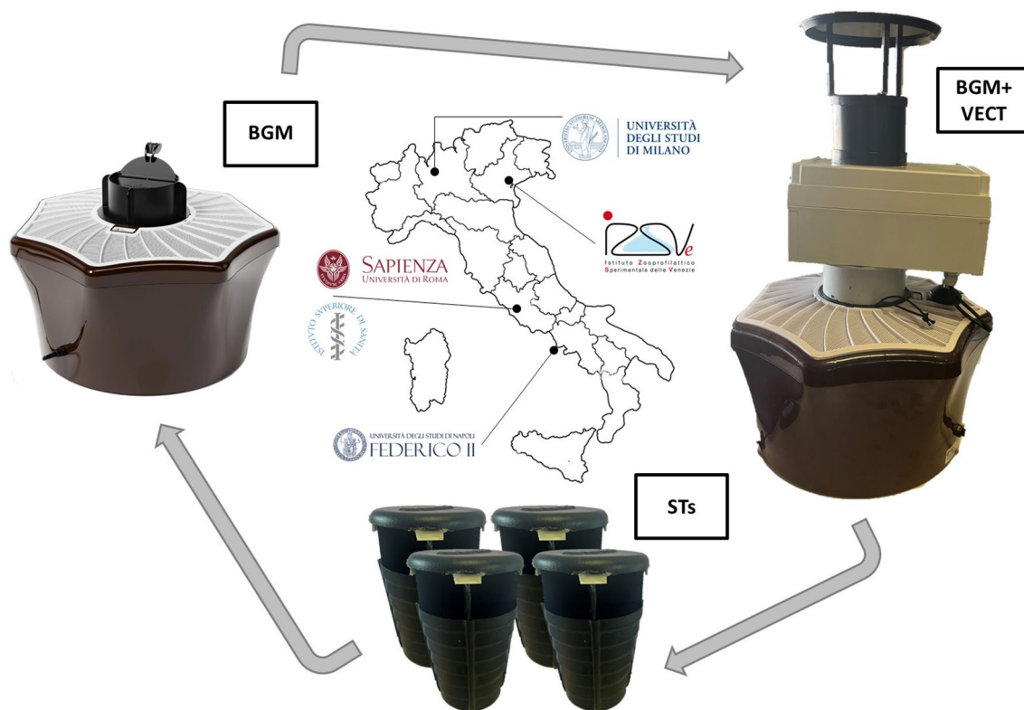
Fig. 1 Experimental design of VECTRACK testing in Italy. Three types of traps were compared: BG-Mosquitaire (Biogents AG; BGM); BG-Mosquitaire equipped with the VECTRACK sensor (Irideon SL; BGM+VECT); four sticky traps (STs; [26]). Each trap was located in one site and moved to a close site (100–400 m) after 48 h following a predefined order of rotation. The complete trap rotation was performed in 6 days. Two additional replicates were conducted in the following weeks in each study area. The same experimental design was implemented in four regions (black dots in the map): Lombardy (by the University of Milan), Veneto (by the Istituto Zooprofilattico Sperimentale delle Venezie), Lazio (by the Sapienza University of Rome and Istituto Superiore di Sanità) and Campania (by the University of Naples Federico II)
