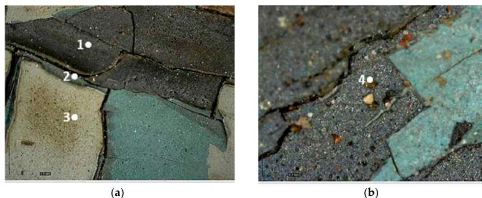
Figure 7. Optical microscope images of the cart's stratification. (a) Image collected at 50× magnification in which the dark grey (1), greenish grey (2), and light grey (3) layers are visible; (b) Image collected at 200× magnification where the deposited particulate is present (4).
