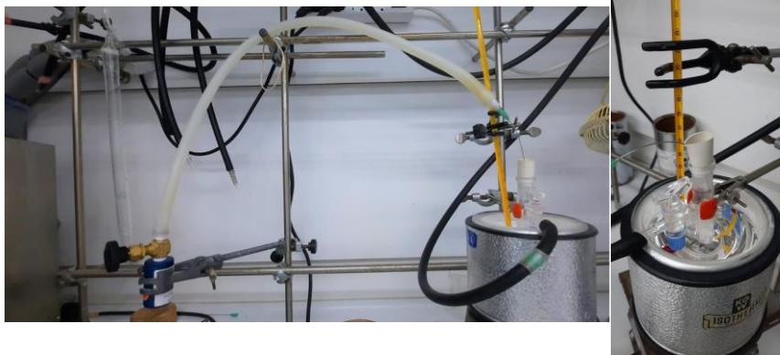
Figure 5.4 Setting up the trifluoromethylation reaction. Left: general setup used to condense \text{CF}_3\text{I} gas in the Schlenk tube. Right: zoom of the reactor cooled to condense the \text{CF}_3\text{I} .
