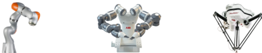
Figure 1.1. Examples of robot manipulators. Starting from the left, the KUKA LBR iiwa robot, the ABB YuMi - IRB 14000 robot and the ABB IRB 360 FlexPicker robot.
