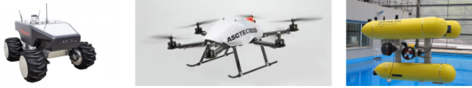
Figure 1.2. Examples of mobile robots. Starting from the left, the Robotnik SUMMIT-XL as representative of the land-based mobile robots, the AscTec Firefly for the air-based and the Girona 500 AUV for the water-based.
