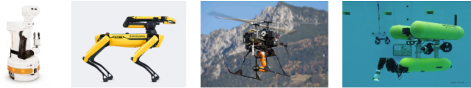
Figure 1.3. Examples of mobile manipulators. Starting from the left, the TIAGo mobile manipulator, the Spot quadruped equipped with a robotic arm, a Fletcher double-rotor helicopter equipped with an LWR arm and the Girona 500 AUV equipped with a manipulator.
