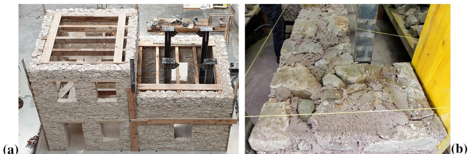
Fig. 1 Physical model: a General view and b Masonry geometric bond pattern (Tomić et al. 2019)
