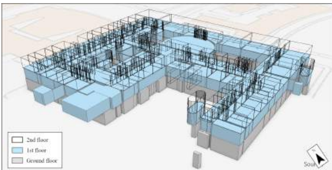
Figure 15. The ground and first floors of the Faculty of Letters and Philosophy obtained by extrusion process and the second floor “schematised” to be internally visualisable in an ArcGIS Pro 3D scene. Authors' elaboration.
