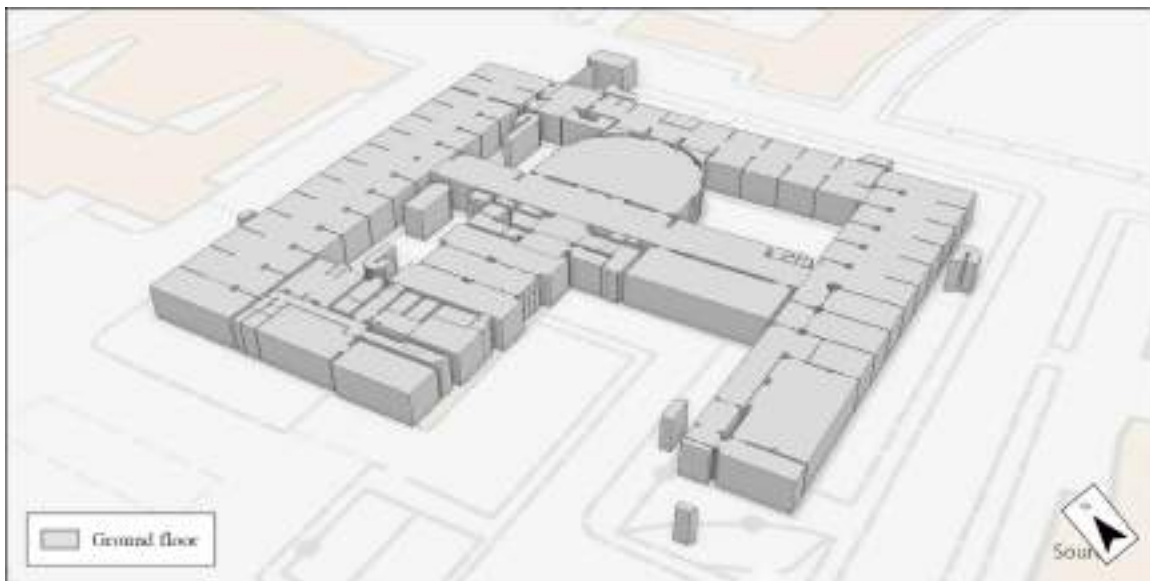
Figure 14. The ground floor of the Faculty of Letters and Philosophy obtained by extrusion process in an ArcGIS Pro 3D scene. Authors' elaboration.
