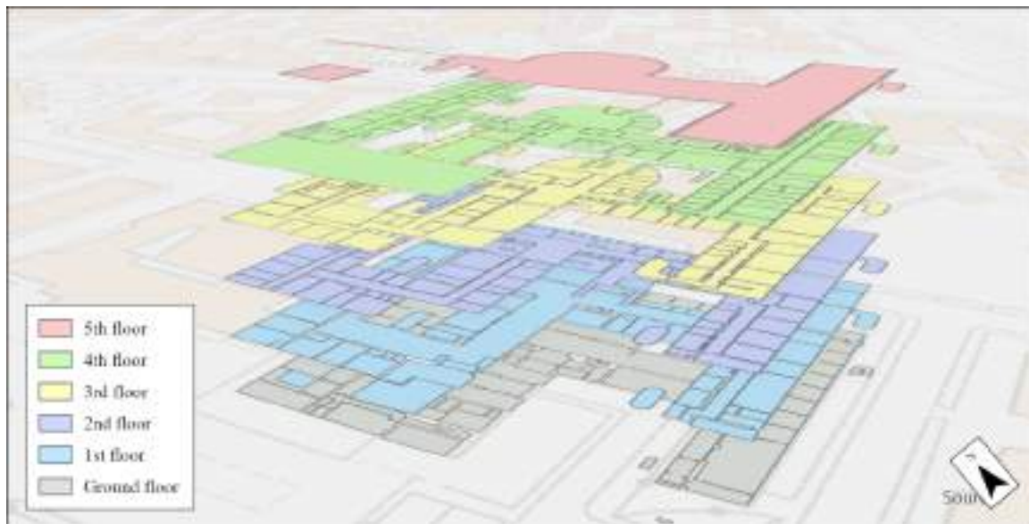
Figure 13. The six floors of the Faculty of Letters and Philosophy, georeferenced and overlaid in an ArcGIS Pro global scene. Authors' elaboration.
