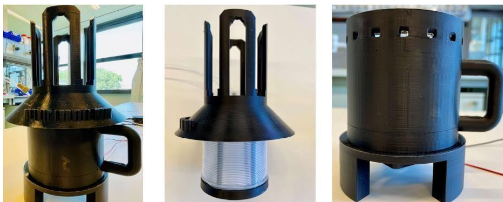
Figure S3. Overview of the 3D-printed flow reactor: left: overall reactor; middle: inside of the reactor (flow loop) and holder for the Kessil lamp in the center; right: main body, internally coated with reflective tape. A fan is mounted on the bottom to keep the temperature stable around 30–33 °C.
