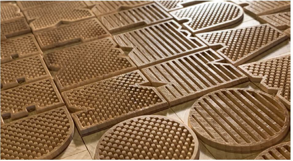
Figure 10. Ryan Molloy, materialization: digitally designed typefaces for letterpress, produced with a CNC milling machine (Hamilton Wood Type and Printing Museum).
