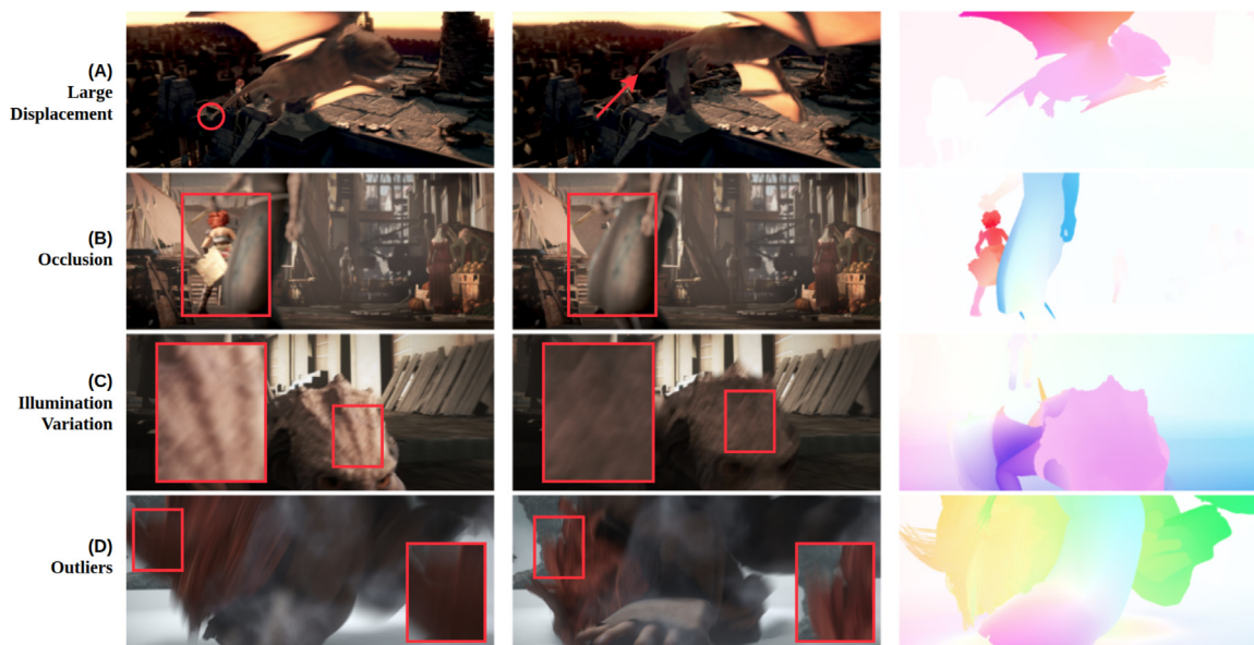
Fig. 4. Representation of some challenges faced during optical flow estimation on the MPI-Sintel benchmark (Butler et al., 2012), with actual ground truth provided. (A) Large Displacement: Fast-moving objects causing displacements, creating difficulties in finding correspondences. (B) Occlusion: Objects in the scene blocking each other, leading to missing or ambiguous flow information. (C) Illumination Variation: Changes in lighting conditions affecting the consistency of flow estimation. (D) Outliers: Presence of motion blur and fog potentially introducing noise and inaccuracies in flow calculation.
