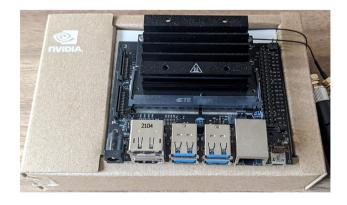
Fig. 8 NVIDIA Jetson Nano embedded board
