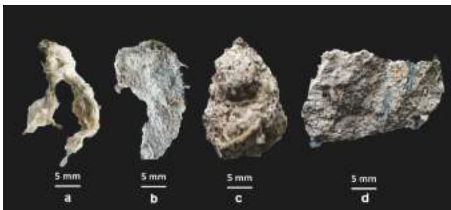
Fig. 3. RGB colour images of the acquired ACM samples used for calibration dataset, composed of: (a) chrysotile rope, (b) chrysotile and crocidolite in a cement matrix, (c) amosite in a cement matrix and (d) chrysotile and crocidolite in a cement matrix.
