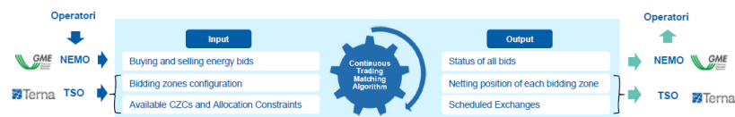
Figure 2.4. Summary of how the SIDC algorithm works.
