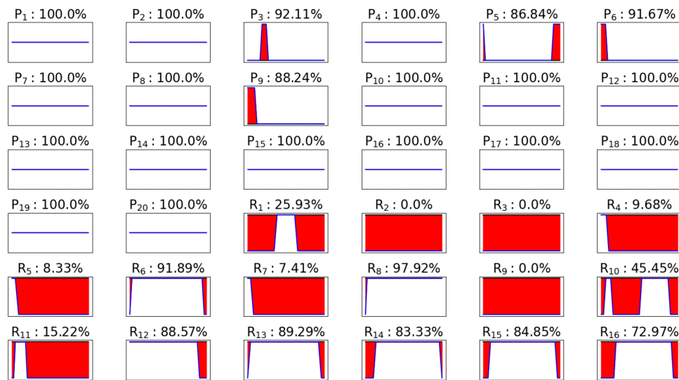
Figure A.4. The rock classifier's performances on the 36 contacts of our test dataset. Each plot corresponds to a separate contact, either plain P_i or rough R_i , and shows a comparison of the ground truth and the predicted class for the entire duration of the contact. When the prediction and the ground truth do not coincide, the gap is filled in red to highlight the error. Although the misclassification rate increases for rough contacts, the overall accuracy on the test set, i.e., the average of the per-contact accuracies labeling each plot, reaches 78%.
