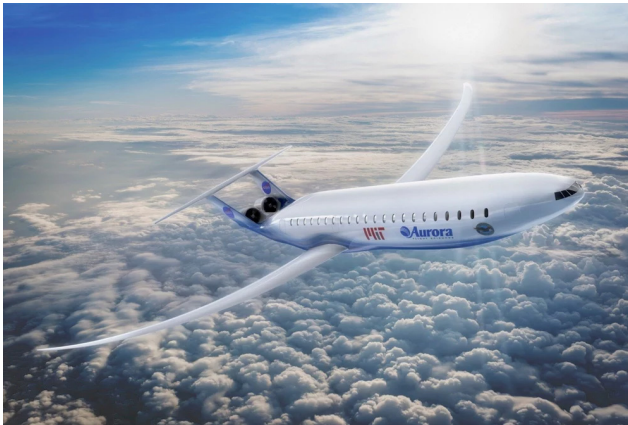
Figure 1.1. Double bubble D8 aircraft design concept, using boundary layer ingestion. Credits: NASA/MIT/Aurora Flight Sciences.
