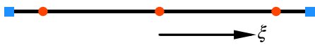
Figure 3.1. One-dimensional standard element at polynomial order p = 2 , with associated solution points (red \circ ) and flux points (blue \square ).
