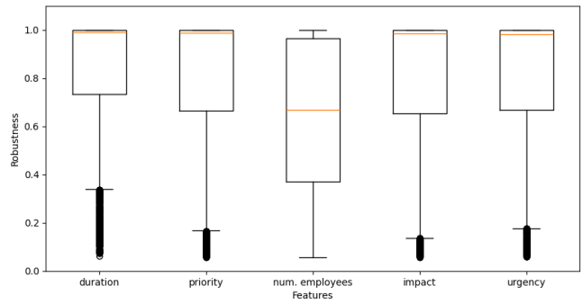
Figure 8: Robustness distribution analysis with the presence of noise for the different IMP log features of the ETR assessment model.
