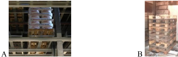
Fig. 3. A Flour stack used for the real-scale test (total weight 850 kg). B Wood pallets used for the real-scale test (total weight 250 kg)
