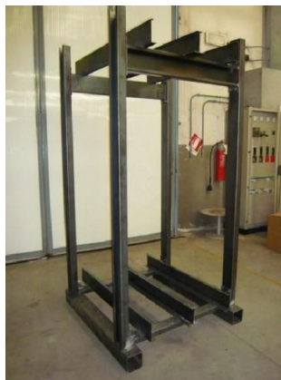
Fig. 10. Steel structure used to contain the food stacks.
