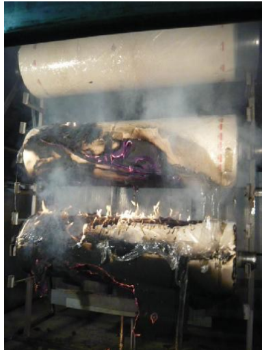
Fig. 7. Cotton rollers after the real scale test (starting from below: roller 1, 2, 3)
