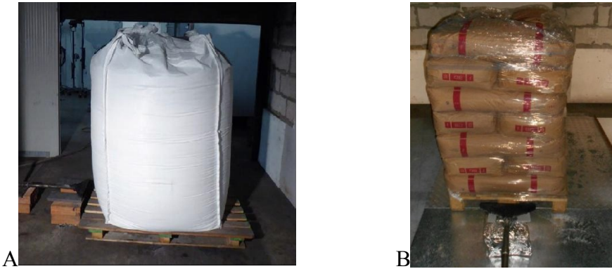
Fig. 4. A: Polypropylene bag containing 1000 kg of sugar. B: Stack of 21 sugar sacks (total sugar 1000 kg)
