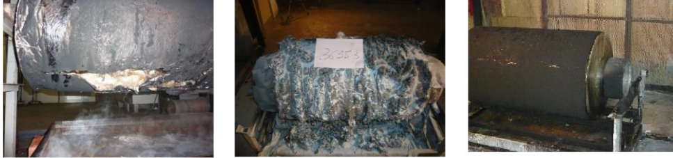
Fig. 8. Polymer rollers after the real scale test (from left to right: polyethylene, polyester, mixed)
