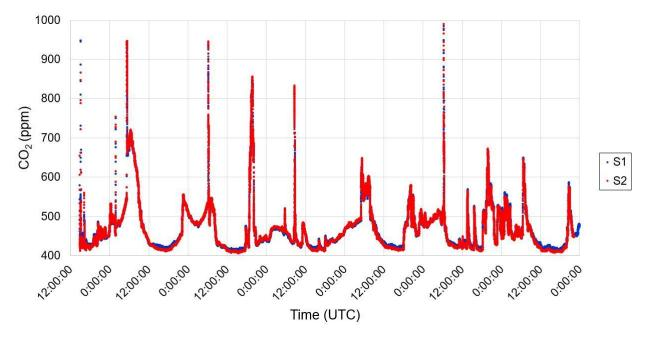
**Figure 2.** Temporal trend of CO<sub>2</sub> concentration during a week-long test to compare the sensitivity of two sensors (different colours).
