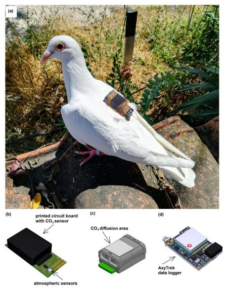
**Figure 1.** Photograph of the device attached on a homing pigeon (a), schematic view of printed circuit board with  $CO_2$  and atmospheric sensors (b),  $CO_2$  sensor (Senseair Sunrise, Senseair AB, Delsbo, Sweden) with the gas diffusion area represented by the white membrane (c), and AxyTrek data logger (d).
