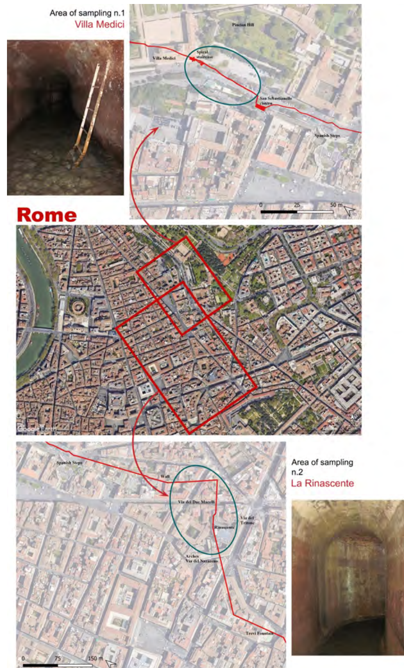
Figure 2. Map of the areas of sampling and photos of the inner duct of Aqua Virgo . Satellite images are taken from Google Earth and QGIS elaboration of Aqua Virgo path using ACEA Ato2 topographical survey, the reconstructive hypothesis of the route of Aqua Virgo presented by Montalbano [26] and new data obtained from speleological investigations inside the channel (Gruppo Speleo Archeologico Vespertilio).
