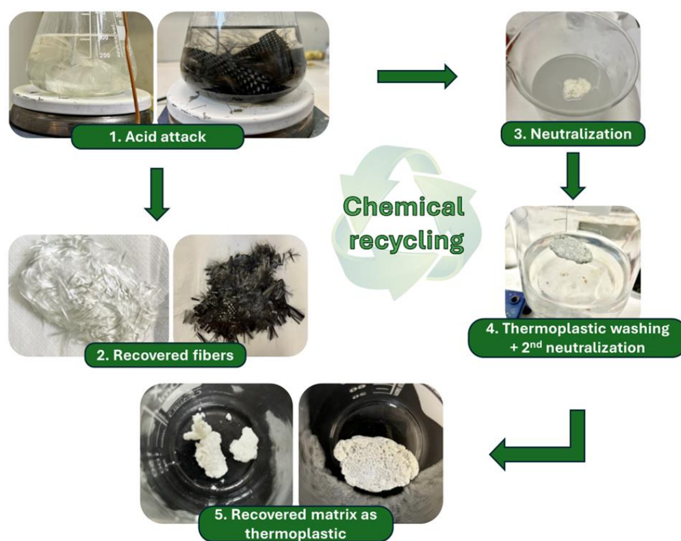
Figure 4. Schematization of the chemical recycling process.
