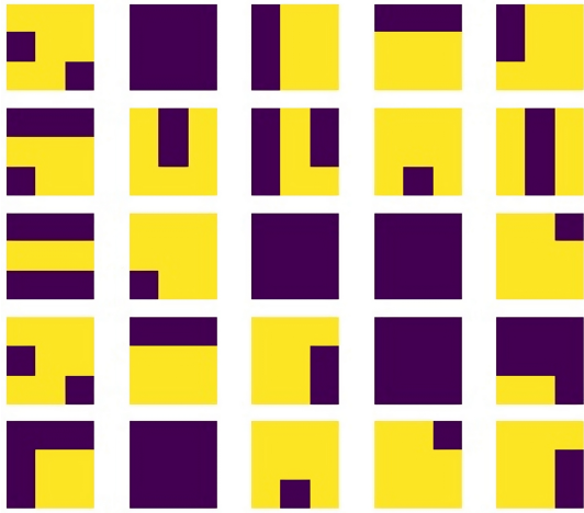
Fig. 2. Illustration of pruned and unpruned parameters within a layer of a 70% sparse MobileNet V2 network. Each 3 \times 3 matrix depicts a channel of the layer's weights. Within each filter, the pruned parameters are shaded in a darker tone, whereas the unpruned parameters are highlighted in yellow.
