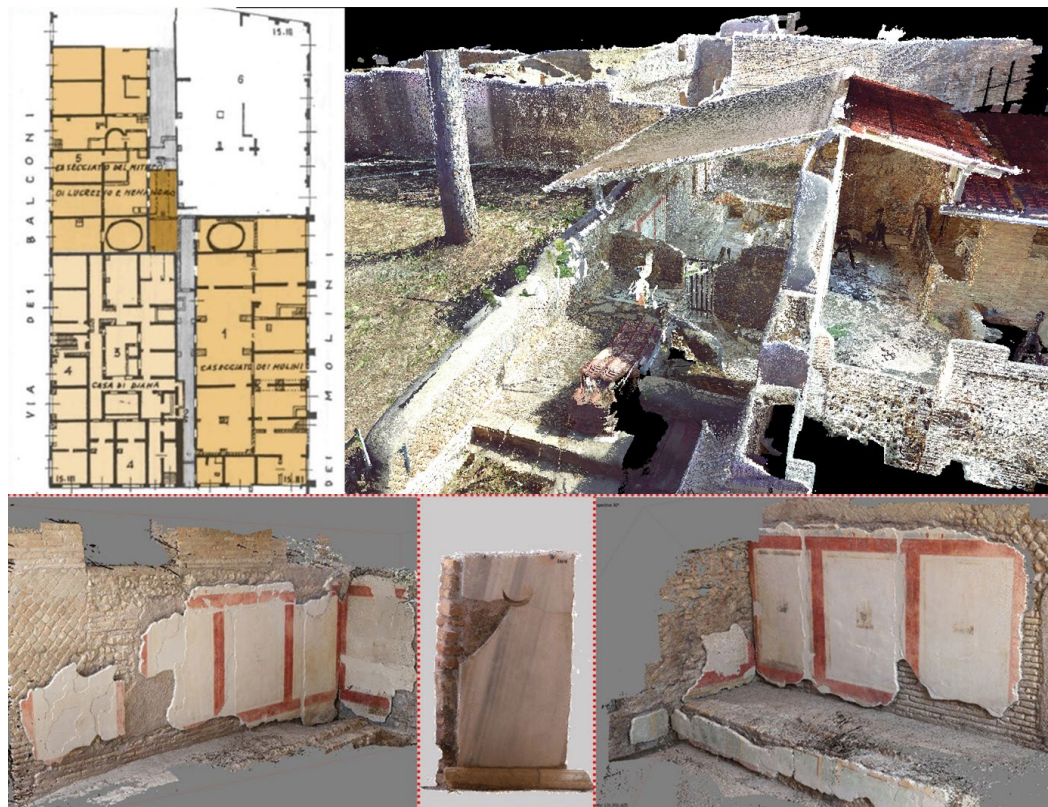
Fig. 1. Mithraeum of Lucrezio Menandro, integrated massive survey, top point cloud generated by 3D laser scanner; bottom SFM of the Mithraeum details.
