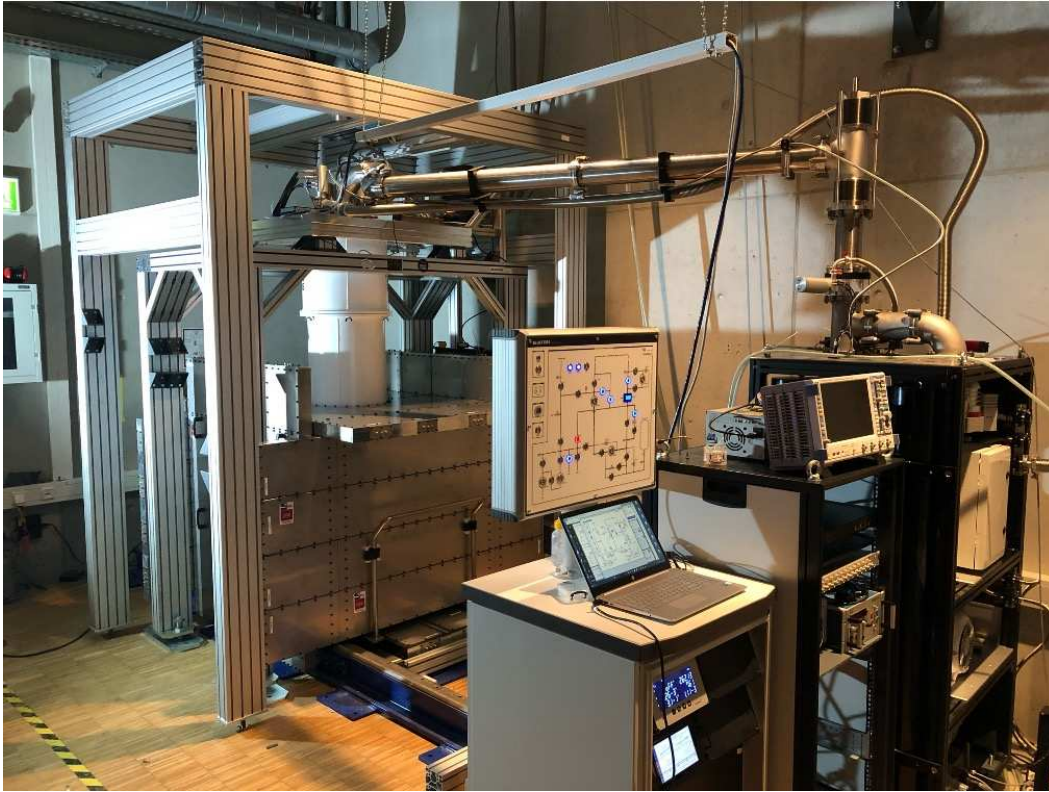
Figure 2.6. Picture of the nucleus cryostat deployed at the Underground Laboratory (UGL) in TUM for the commissioning and background run before the move to the Chooz nuclear power plant. In the picture, the gas handling and cryostat monitor electronics is shown along with the cryostat with its rack surrounded by the room temperature shields and muon veto.
