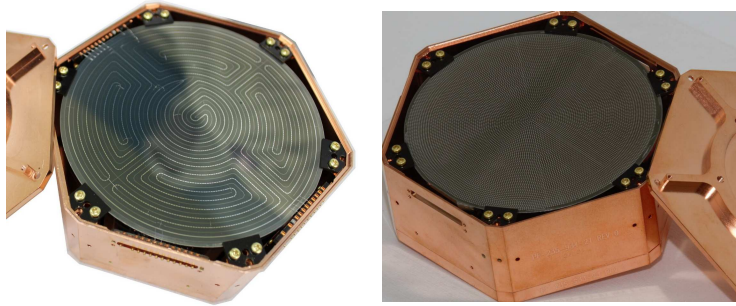
Figure 1.27. Detectors employed by the MINER experiment: left: double readout detectors, right: high voltage phonon detector based on the Luke effect. Figure from [57].
