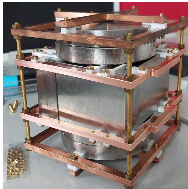
Figure 2.12. COV mockup crystals, made of silicon, installed in the holding copper cage structure for mechanical tests.
