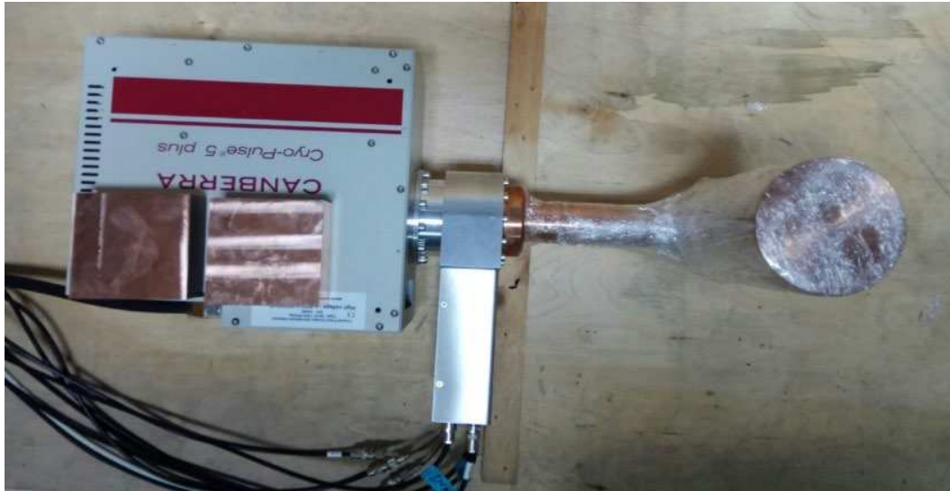
Figure 1.23. Electrocooled HPGe detector from the TEXONO collaboration (figure from [49]).
