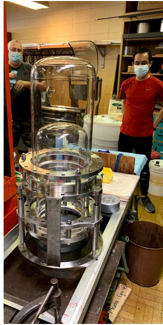
Figure 1.28. Case of the LAr bubble chamber deployed by Pico (figure from [59]).
