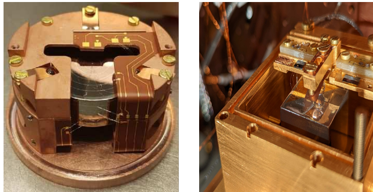
Figure 1.26. Detectors developed by the RICOCHET collaboration. Left: Cryocube detector (figure from [54]). Right: Q-array prototype detector (figure from [55]).
