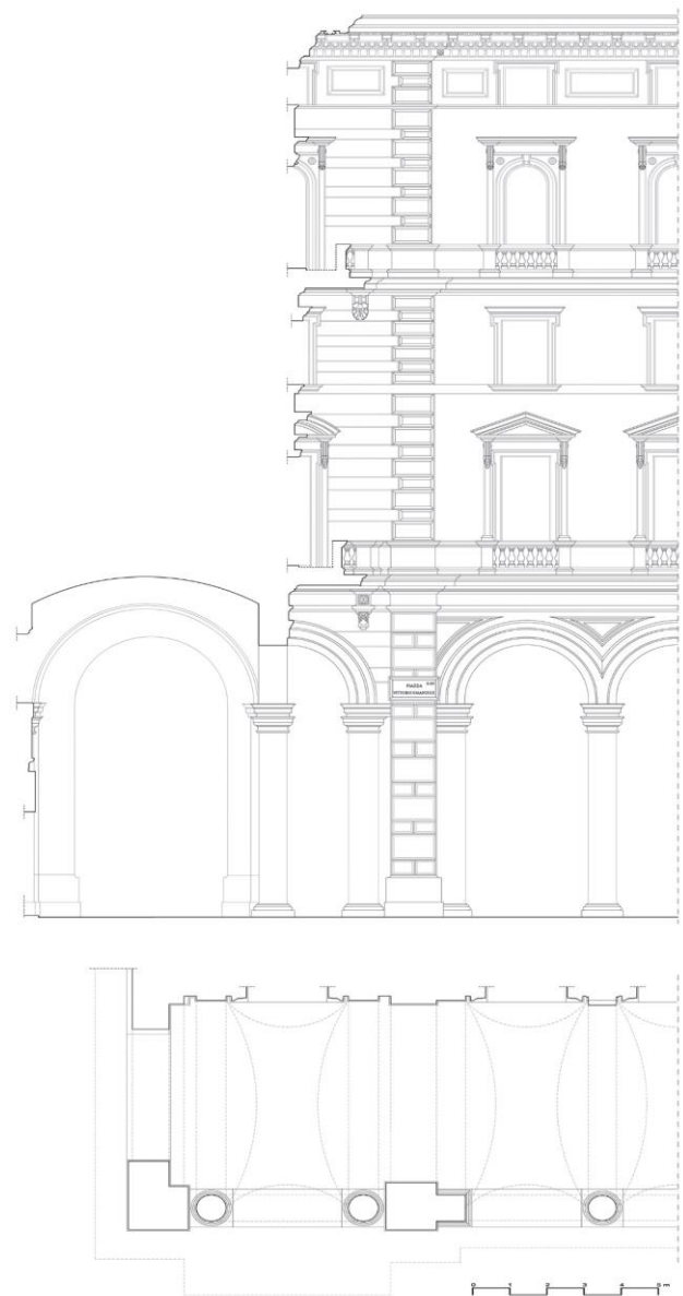
Fig. 21: Detail of section, elevation and plan of the corner bays of block XXV (authors' elaboration).
