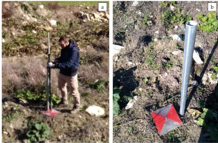
Figure 4.5. a) An operator during GNSS-RTK data collection. b) A self-made GNSS target.
