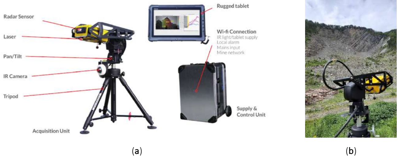
Figure 2.3. (a) HYDRA-G equipment; (b) Terrestrial ArcsSAR Interferometry installed at PBL.
