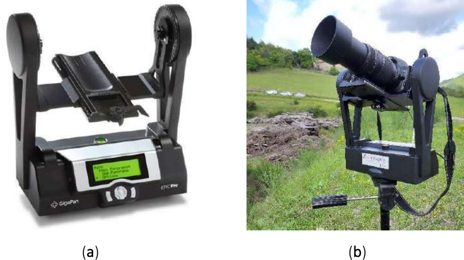
Figure 2.2. GigaPan acquisition system used at PBL: (a) GigaPan robotic head with screen and controls; (b) GigaPan system equipped with a Nikon D5000 camera and 300mm telephoto lens.
