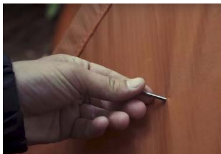
Fig. 14 Holes and punctures can be repaired when combined with the special double-sided coating and heat from fingers [8]
