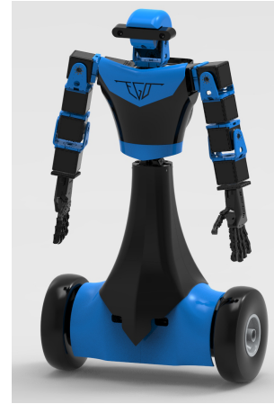
Fig. 1. ALTER-EGO, a prototype WIP robot developed at the University of Pisa [7].
