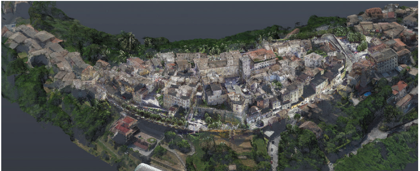
Figure 9. Point cloud automatically integrated between TLS and UAV based on shared coordinates.
