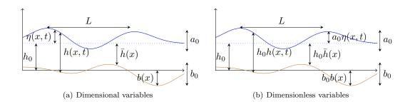
Figure 1: Water waves: notation
