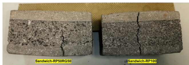
Fig. 10. Failure modes of sandwich composites.
