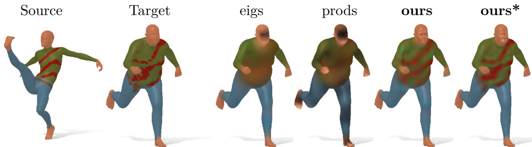
Figure 1.19. RGB signal transfer comparison on a pair from the SHREC'19 dataset. Our approach better transfers the fine details. In this example, the noise in the ground truth correspondence due to wildly different meshings is enough to produce local distortion in the function transfer, but our approach remains stable and produces a smooth correspondence.
