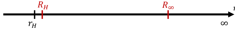
Figure 2.3: The boundary conditions are imposed at the numerical values for the horizon R_H and for infinity R_\infty to avoid numerical divergences.
