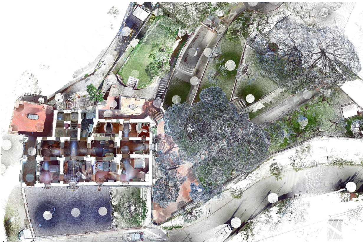
Figure 14. Plan view of the point cloud from the laser scanner survey. Station points are clearly visible.
