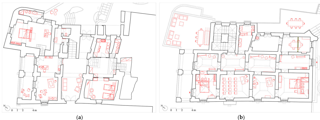
Figure 19. Villa Murat converted into Artists’ residency. (a) Ground floor plan; (b) first floor plan.
