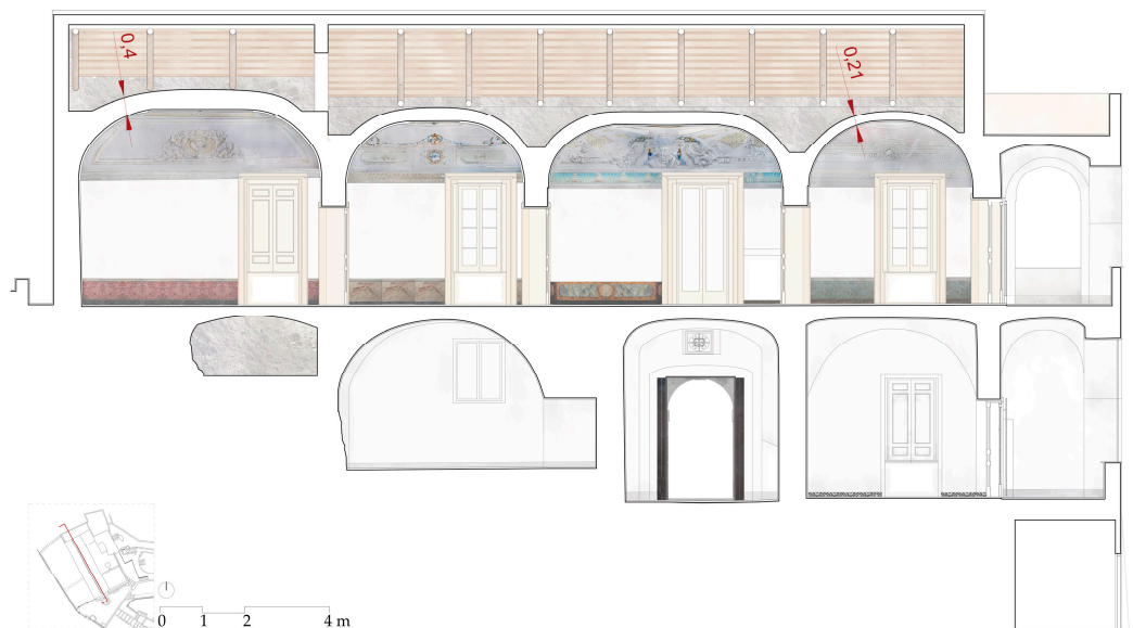
Figure 17. Longitudinal section. The differences in the thickness of the vaults are evidenced. The part of the roof on the left of the section is that with trussing structures instead of trusses.
