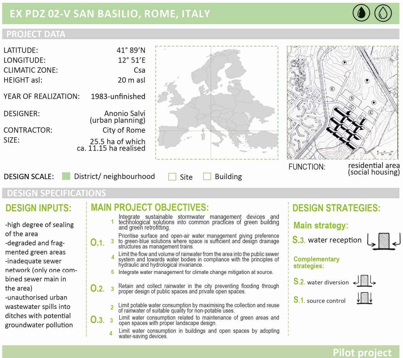
Figure 10. Pilot project area in San Basilio, Rome: A Summary of project data, inputs, and results from applying the objectives–strategies–solutions matrix for sustainable stormwater management (SWM). Design strategies are represented using icons defined by the Authors; the direction of the arrows indicates the adopted water management approach. The original urban plan included areas designated for residential buildings (E), public services (S), commercial functions (C), and park areas (tree symbol), as shown in the figure, which were never implemented.
