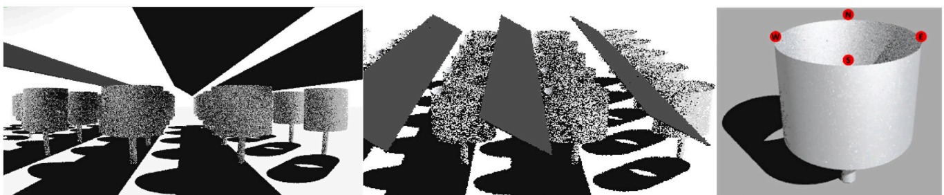
Fig. 2. Modeling of an Agrivoltaic system with olive trees using Bifacial Radiance Raytracing Tool. Scene created to obtain the incident radiation in different points.
